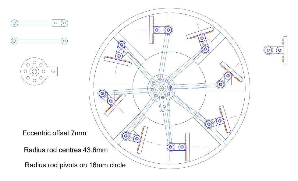
Wheel, hub and eccentric assembled with 10BA brass screws into tapped holes
